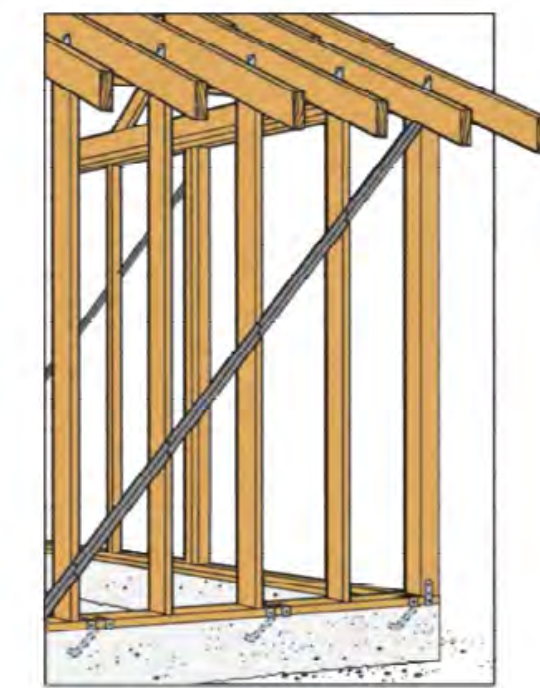
FIGURE 5B—TYPICAL TWB (T-TYPE) EXTERIOR WALL BRACE INSTALLATION (MAXIMUM 3/8-INCH DEEP SAW KERF IN STUDS)
